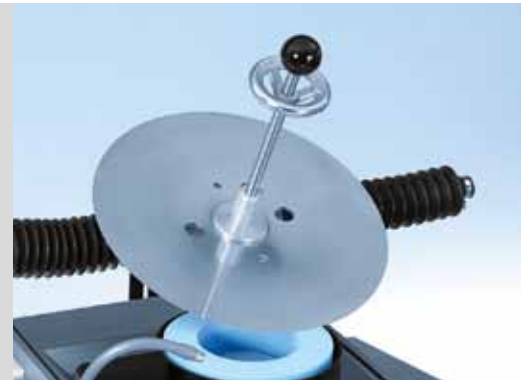
Circular knives (diameter 80-480 mm) sharpened with the cup grinding wheel
