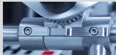
Locking mechanism used to change knives
