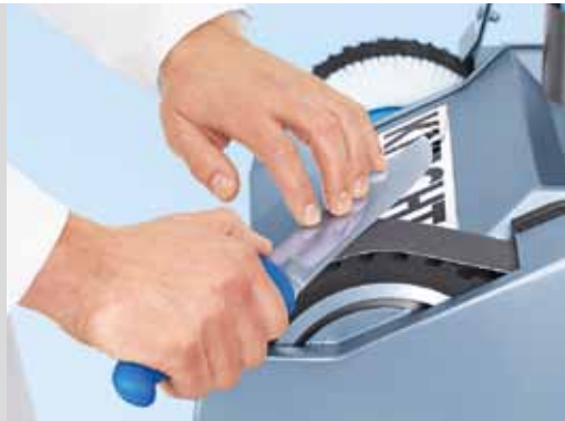
Sharpening hand knives on the wet-grinding belt
